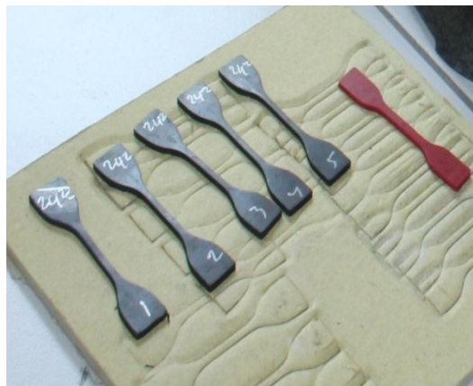
Gambar 1. Sampel uji dumbbell
